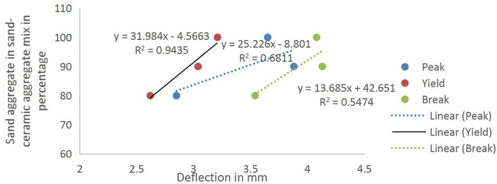
Figure 15: Aggregate mix ratio and deflection nexus
