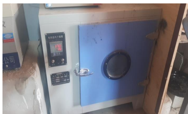
Figure 3: Electric blast drying oven
