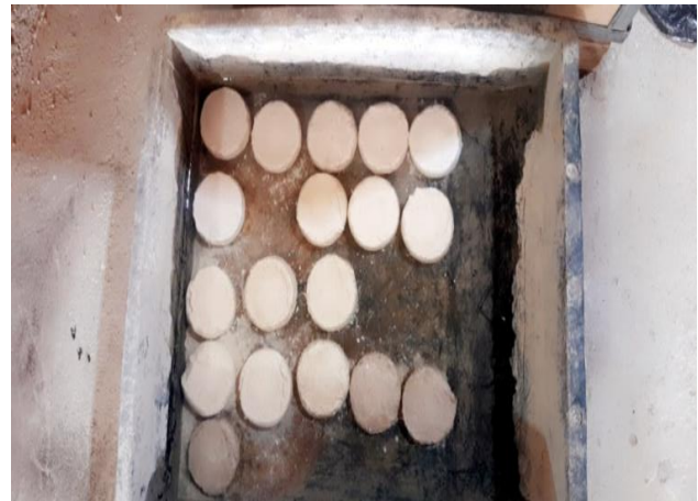
Figure 5: Samples being Soaked
