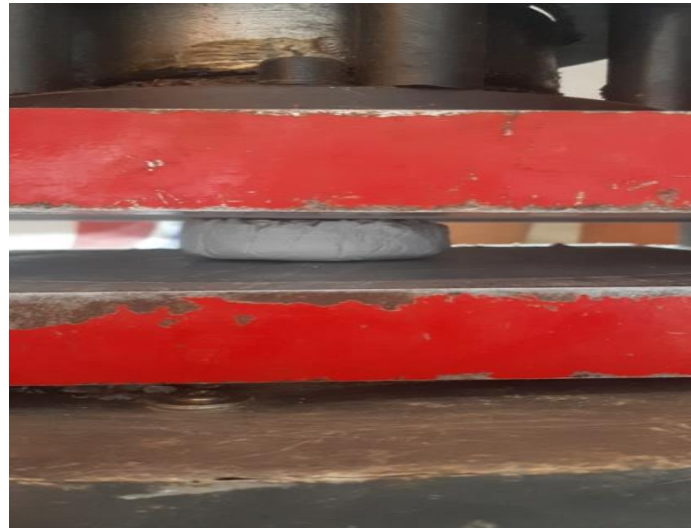
Figure 6: Sample loaded to the press jaws
