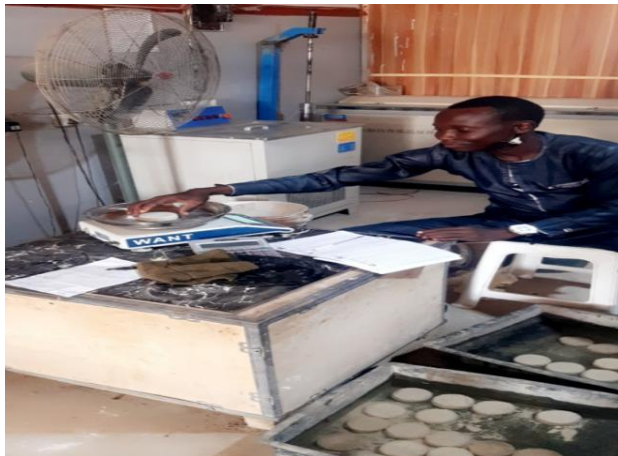
Figure 4: Samples weighed for Porosity
