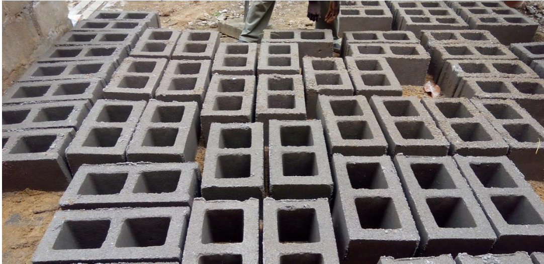
Figure 3: Metakaolin sandcrete blocks produced at various replacement levels
