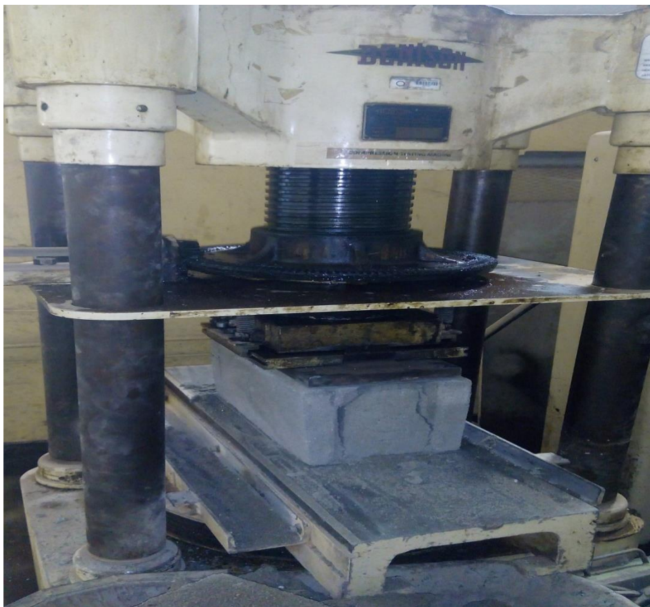
Figure 4: Crushing Strength of MKSB by Universal Compression Machine
